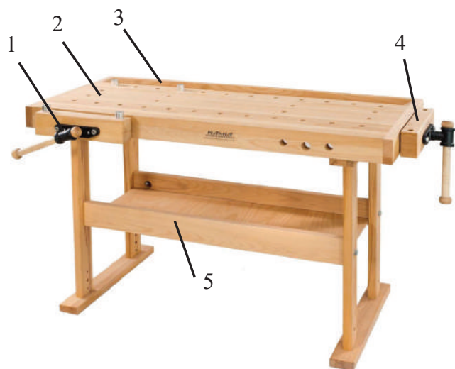
6-rasm. Duradgorlik dastgohi tuzilishi:
