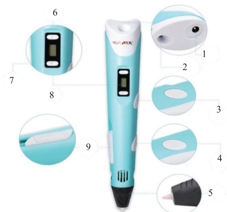
103-rasm. Issiq 3D ruchka tuzilishi: 1 – quvvat manbayi; 2 – plastik sim teshigi; 3 – plastik simni orqaga qaytarish tugmasi; 4 – plastik simni oldinga o‘tkazish tugmasi; 5 – ishchi qismi; 6–7 – haroratni rostlash “+”, “–” tugmalari; 8 – LED ekran, 9 – tezlikni rostlash tugmasi.
